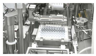
Cartridge in process control (weight check) on a groninger line
