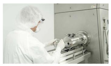
Docking a Beta Canister on an MTI (Material Transfer Isolator) from SKAN
