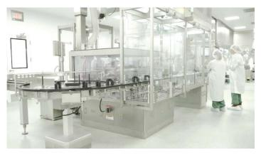
Groninger vial filling line with SKAN isolator, branded integra
