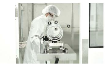
Docking a Beta Canister on an MTI (Material Transfer Isolator) from SKAN2
